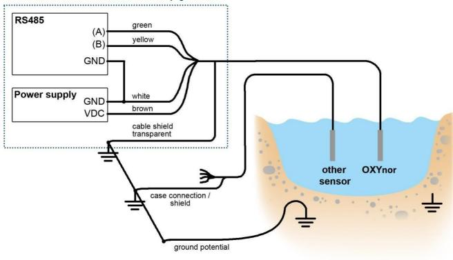
In general, the connection between the ground conductors should be as short as possible. A grounding bar directly after the water tanks, connecting the grounds of different sensors improves the grounding quality.
